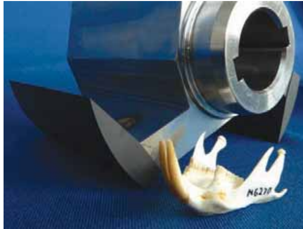
Self-sharpening cutting tools and their biological inspiration (water rat)
