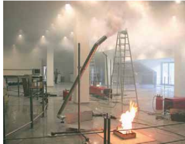
Ceiling smoke layer in a multi-purpose area
