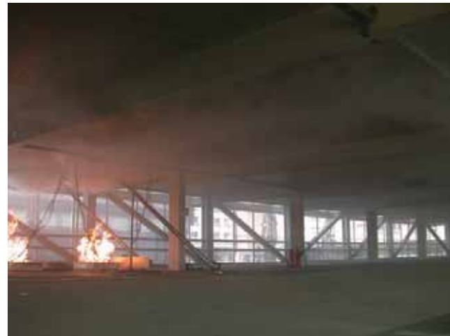
Hot smoke test in a multi-storey car park
